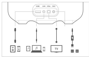
**Service**: The USB port is used for firmware upgrade or Wi-Fi set up only and will not charge attached devices.
