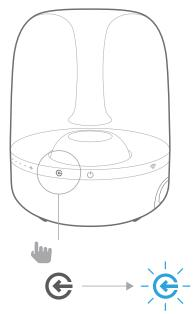
Use the device's Bluetooth pairing menu to pair it with the Harman Kardon Aura. The unit will appear as HK Aura BT in the list of Bluetooth available devices. When the Harman Kardon Aura's source button LED illuminates blue constantly, it is paired with the device and you can stream audio via Bluetooth from the device to the Harman Kardon Aura.
